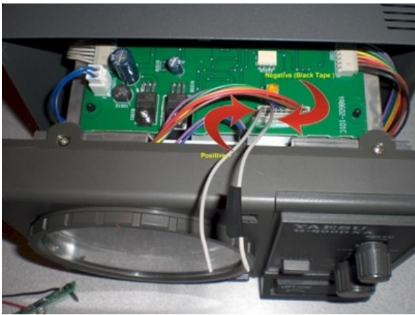
#3 (+ & - to Yaesu Illuminator Board DXA Boxes)
