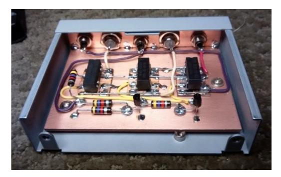
A small metal box, such as an old 5-Port Ethernet Switch would be just about the right size. Cut 3 rectangles of copper clad board and scribe lines with a hobby knife to create 8 properly spaced solder "islands". Glue them to main board. First, a little planning.
