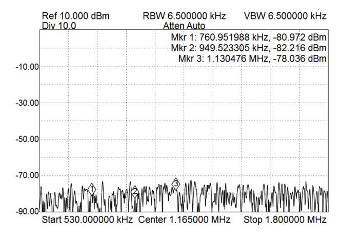
80m dipole through high pass filter to spectrum analyzer input:
