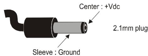
The sleeve is negative, and can be grounded or floated at the power supply. The center pin is positive, and **MUST** be ground isolated. The supply must be capable of supplying 300mA continuous at 12-15 volts dc, when using the standard RCS-10 outdoor relay box. To ensure the supply meets these requirements, we recommend using 500mA or larger power adaptors (“wall-warts”). This unit will accept voltages of 25 volts if you want to use it with other relay systems.
