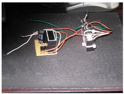
Two versions, one a prototype and another on vector board: It takes a few minutes to make. If you need a longer delay, change the time constant of R1/C1.Parts cost: about \$5.
